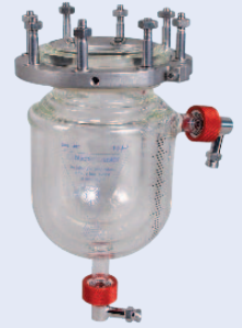
Type 1I Glass vessel with heating jacket and vacuum insulation jacket, without drain valve 0.5 / 1.0 / 1.6 l max. 12 bar / 200°C
