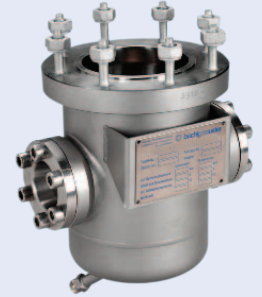
Type 4 Metal vessel with heating jacket, 2 sight glasses and drain valve 1.0 / 1.5 / 2.0 / 3.0 / 5.0 l max. 60 bar / 250°C
