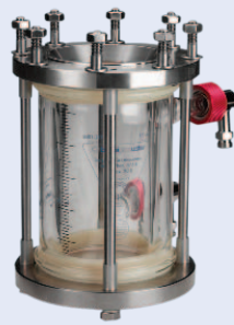
Type 2 Glass/Metal vessel with heating jacket and drain valve 0.5 / 1.0 / 1.5 / 2.0 l max. 12 bar / 200°C
